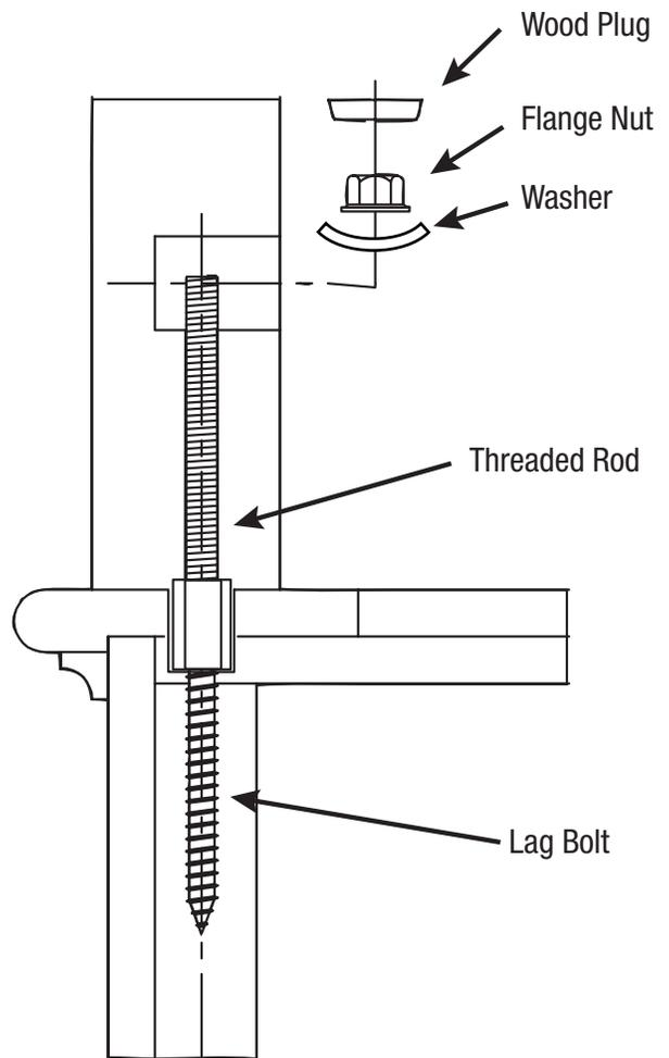
**Tools Needed:** Electric drill with 3/8", 1/2", 1", and 1-1/2" wood drill bits. 5/8" wrench or socket, 9/16" wrench and hammer. Optional- wax to ease installation of lag bolt
