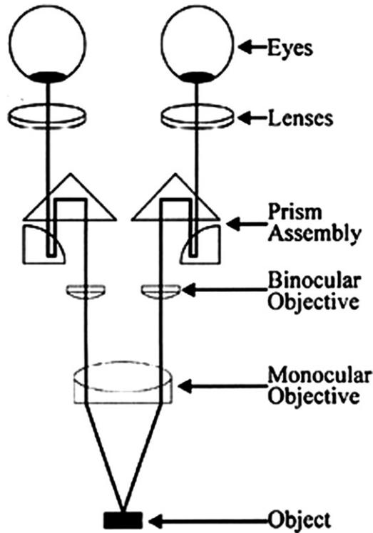
**Fig. 8.** Galilean optics. Parallel optics enables the observer to focus at infinity, relieving eyestrain.
